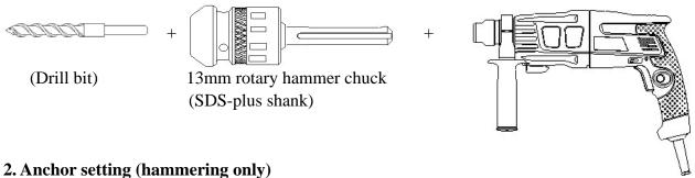
O Anchor setting adapter (for rotary hammer)
