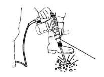
2. Operate this demolition hammer by utilizing extra pressure. The performance will be better if it is pressed properly against the work surface.
