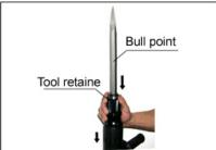
(2) to pull out the bit follow the install procedure in reverse.
